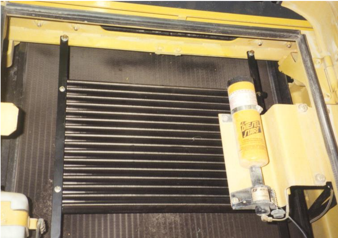
Condenser mounted in location.
